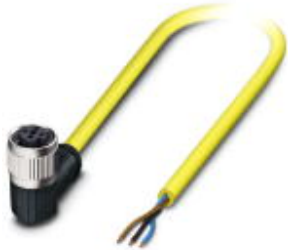
Sensor/Actuator cable, 3-position, PVC, Yellow RAL 1021, Free cable end, on Socket angled M12-SPEEDCON, A-coded, Cable length: 2 m
